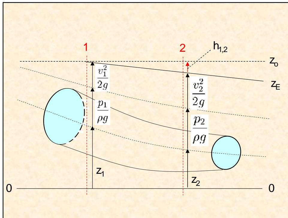
$$\frac{v_1^2}{2g} + \frac{p_1}{\rho g} + z_1 = \frac{v_2^2}{2g} + \frac{p_2}{\rho g} + z_2 + h_{1,2}$$
