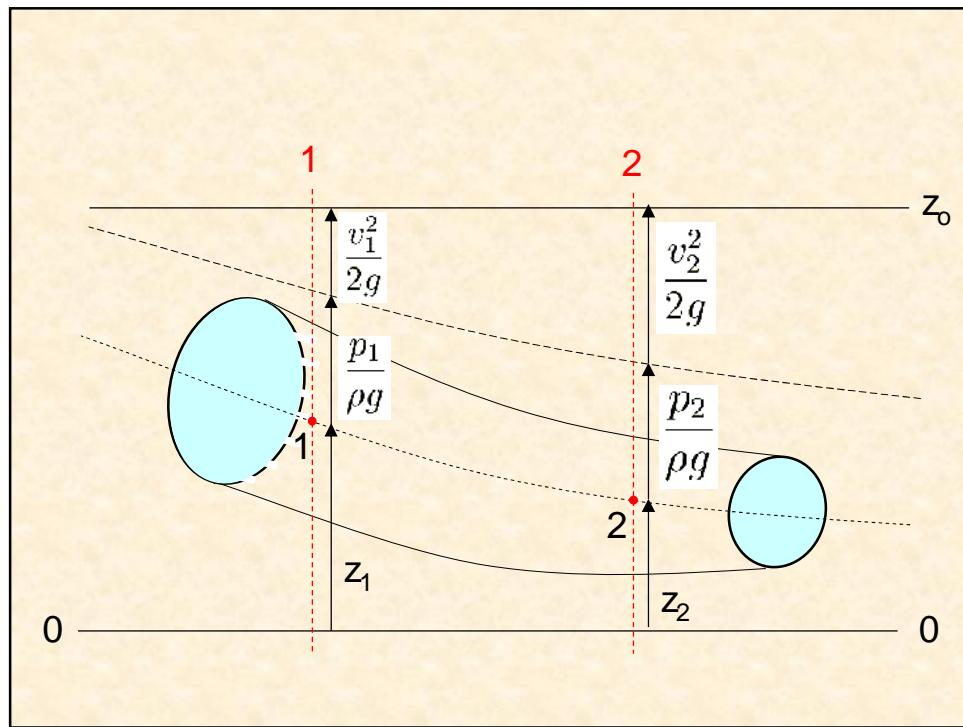
$$\frac{v_1^2}{2g} + \frac{p_1}{\rho g} + z_1 = \frac{v_2^2}{2g} + \frac{p_2}{\rho g} + z_2$$
